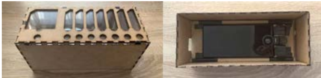
■ Figure 3.2 BrailleBuddy’s original lid consisted of two thin wooden plates. In the new prototype the lower plate was replaced with a see-through acrylic glass layer [91]. This change enables the smartphone’s camera to monitor the game state from below when placed at the bottom of the box.
