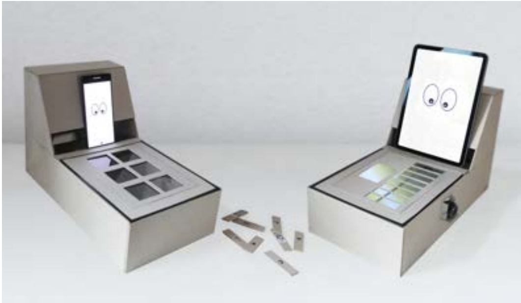
■ Figure 6.1 The Playmake prototype consists of a cardboard box with a see-through playing field embedded in the lid. Exchangeable custom game layouts with slots for designated game elements can be placed on the transparent layer. The setup is suitable for smartphones and tablets.
