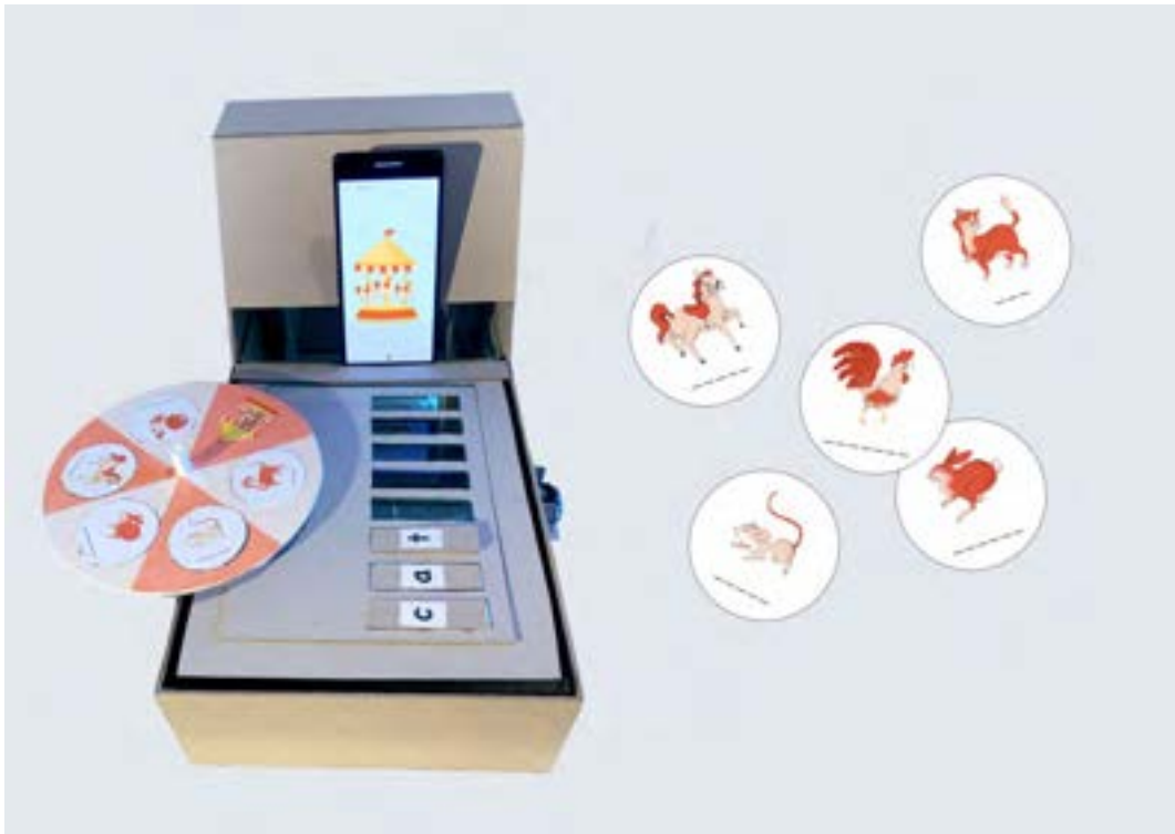
■ Figure 6.7 For the game Spell Carousel [96], we have constructed a rotating cardboard disc on which cards with illustrated images are placed. The goal is to spell the associated words. After a word is solved, the carousel can be spun one position further.
