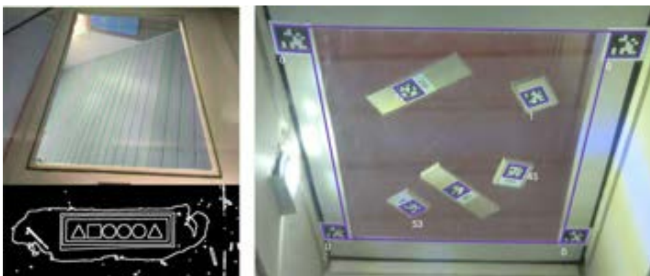
■ Figure 5.2 The left image shows the initial attempt to use edge detection to find the game layout borders and the game element codes. To simplify the process, we utilized AprilTags to achieve both goals, as depicted in the right image.
